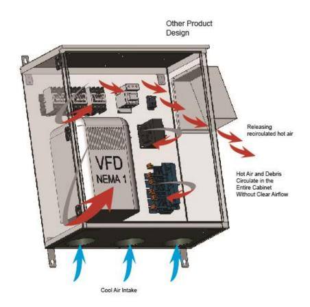
While this is an inexpensive and simple way to cool the VFD system, the downside is air flows directly across the internal electronics and subjecting them to dust, humidity, and debris from the outside air.
