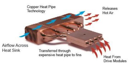
Copper heat pipes transfer localized heat away from sensitive components to heat exchanging fins directly in contact with outside air. Heat is transferred to the circulating air which keeps the VFD operating at a safe temperature.
