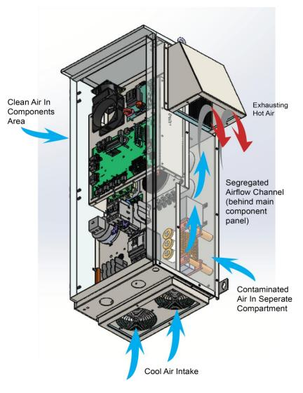
Indirect cooling methods such as air conditioning, copper heat pipes, and water cooling are more effective at cooling and keeping contaminants away from critical electronic components; however, the major disadvantage to these systems is that they are cost-prohibitive, both on the initial installation and with on-going maintenance and repairs.
