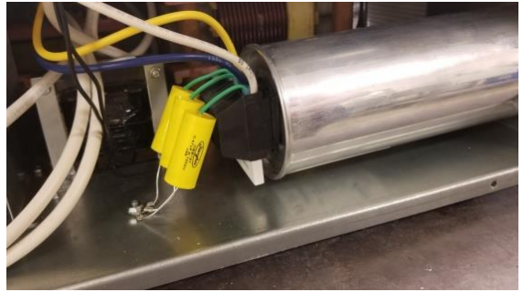
Figure 44 – Line Filter Cap Location – Enterprise Series
