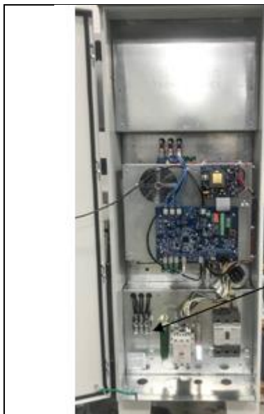
Figure 15 – Signature Series Output Power Terminal Locations
