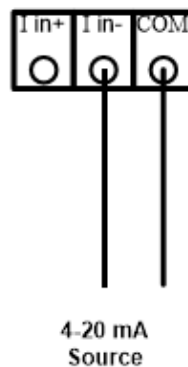
b. 4-20 mA Transducer with External Source
