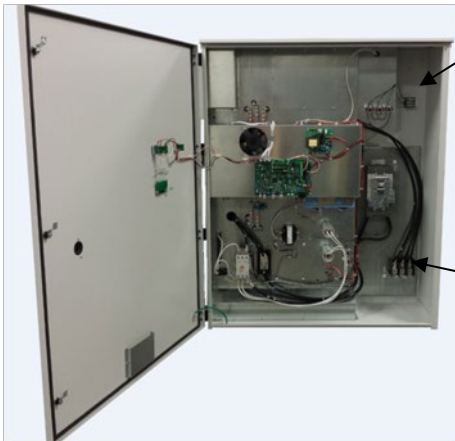
Figure 6 – Performance Series Output Terminal Location
