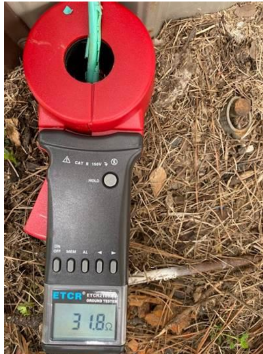
Figure 2 – Earth Ground Resistance Meter. Measured value should be 4 Ohms or less
