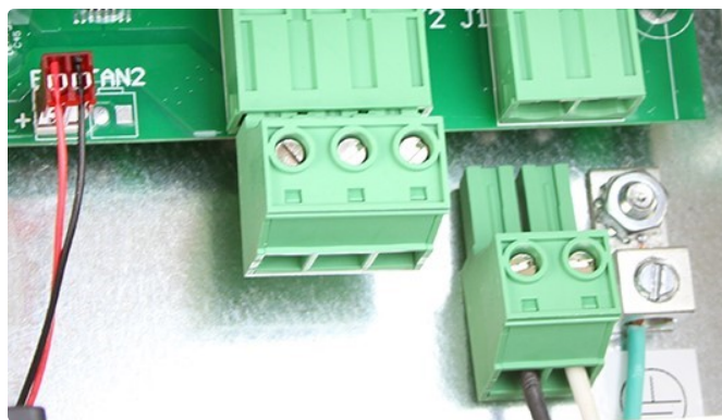
Removable J1 and J2 terminal blocks inside chassis
