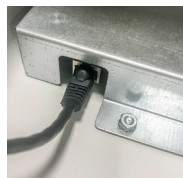
RJ45 cable connected to keypad on underside of front panel. Release cable before removing cover.
