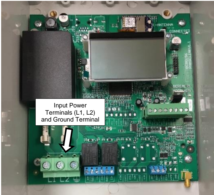
Figure 4 – Input Power Terminal Locations
