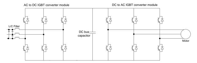
Figure 2 - 3LHX Series Block Diagram
