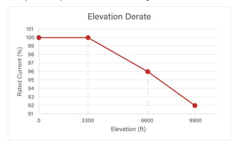
Figure 24 - Elevation Derate Chart
