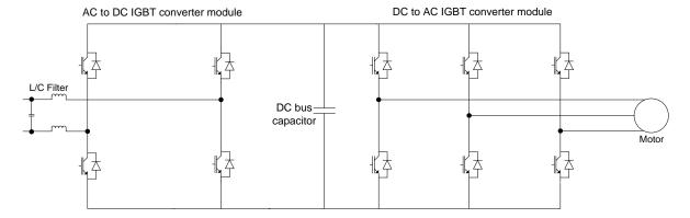
Figure 3 - 1LHX Series Block Diagram
