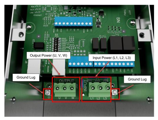
Figure 5 – D1/L1 Frame Size Power Terminal Location
