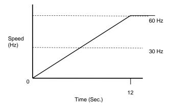
Figure 19 – Start-Up Ramp Time (1.1.13 SUBMERSIBLE PUMP parameter disabled)
