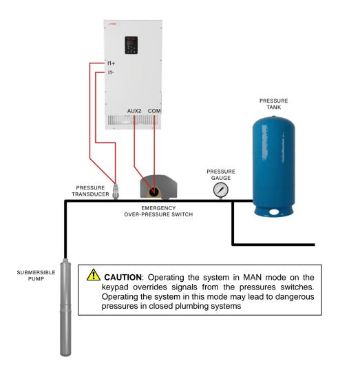
Figure 21 – Analog Constant Pressure One-Line Diagram
