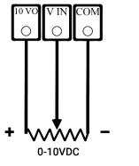
a. Potentiometer Connection Diagram
