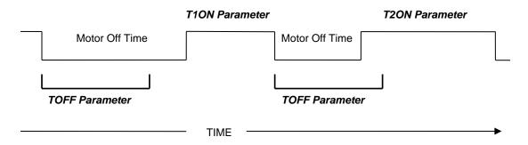
Figure 20 – Motor On and Motor Off Times
