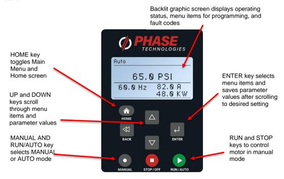
Figure 16 – Keypad and Graphic Display
