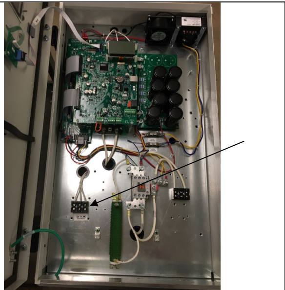
Figure 8 - Enterprise Series Output Power Terminal Locations
