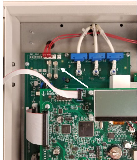
Fuses F1 and F2 are located on the circuit board beneath the display.
