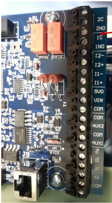
Figure 15 – Programmable Relays for Lead/Lag Control
